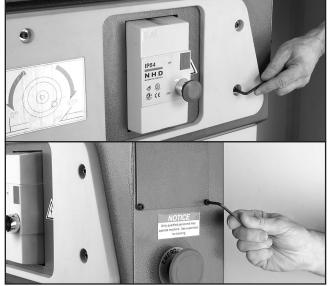
Figure 17. Removing cover plates.
